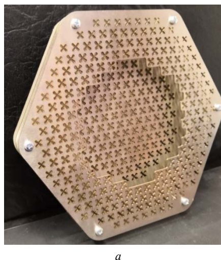
Fig. 7. Schemes of construction for conformal reflectarrays: а – stepwise; б – angular
