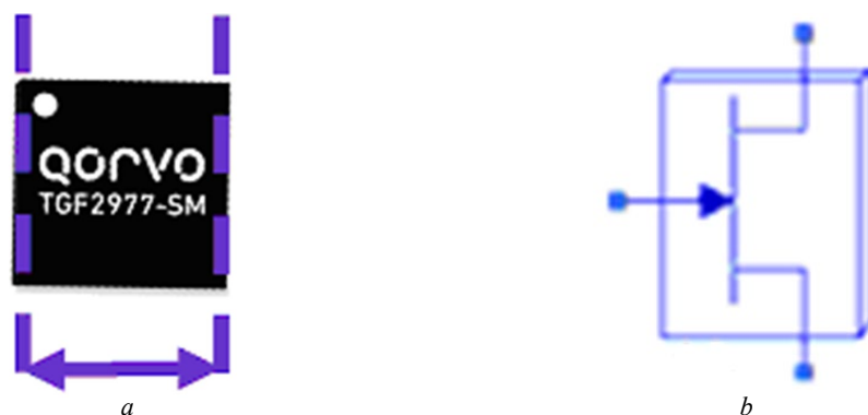
Fig. 2. Reference plane (a) and pins for measurements (after packaging) (b) of HMT-QOR-TGF2977
