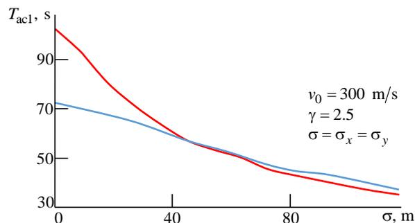
Fig. 6. Dependence of the average object tracking time on the measurement error of coordinates for the proposed algorithm (red line) and known algorithm (blue line)
