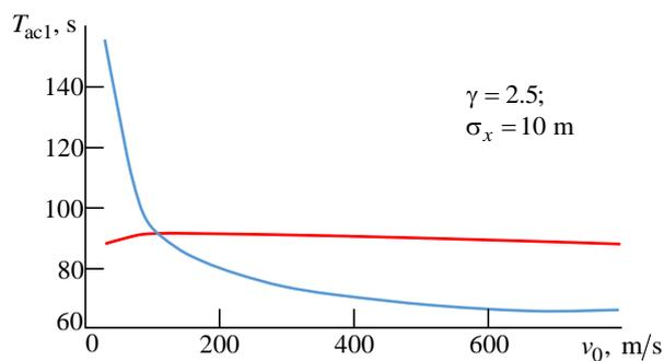
Fig. 7. Dependence of average object tracking time on initial speed for the proposed algorithm (red line) and known algorithm (blue line)
