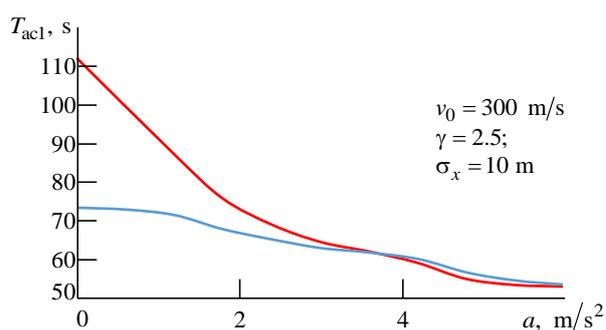
Fig. 8. Dependence of average object tracking time on acceleration for the proposed algorithm (red line) and known algorithm (blue line)
