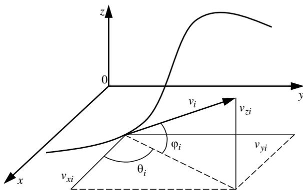
Fig. 1. The specifying of velocity in the body-fixed frame
