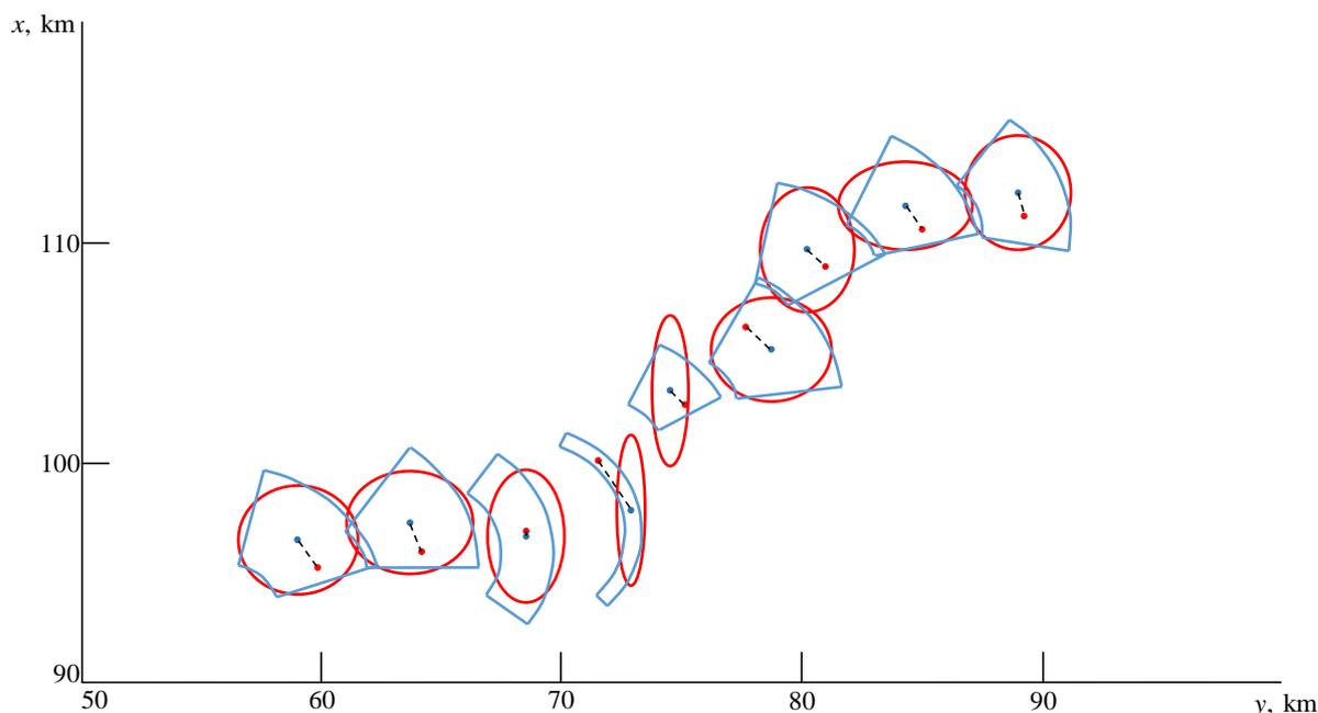
Fig. 4. Position and shape of strobes for maneuvering target.
