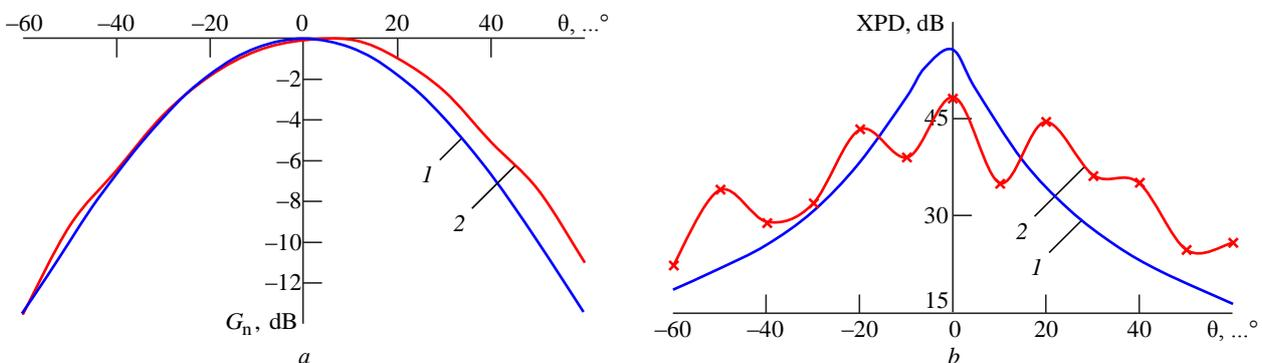
Fig. 12. Theoretical 1 and experimental 2 dependences of the parameters of an elliptical double-ridge antenna at a frequency of 18 GHz in the plane  $\varphi = 45^\circ$ : *a* – normalized to the maximum gain ratio; *b* – XPD
