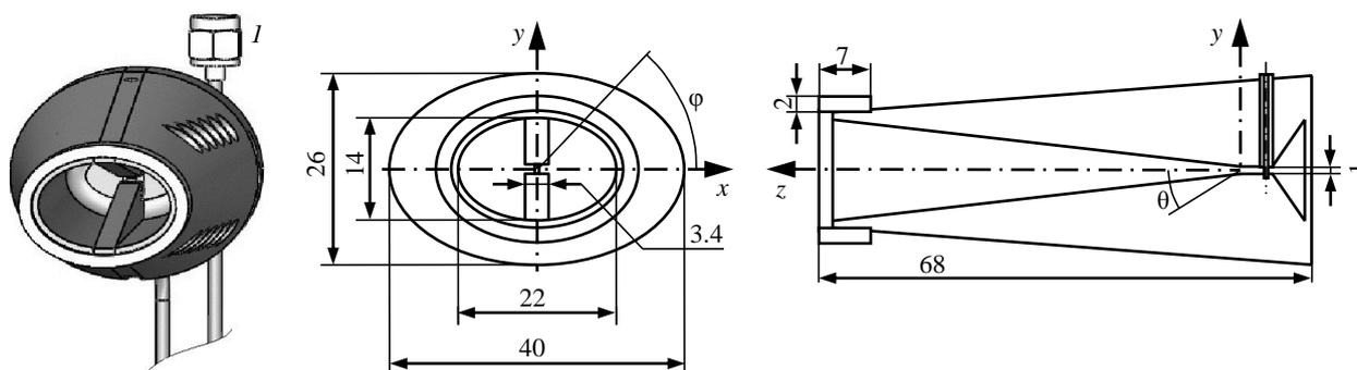
Fig. 8. Model of an elliptical double-ridged antenna: *I* – 50-Ohm coaxial waveguide with fluoroplastic insulator
