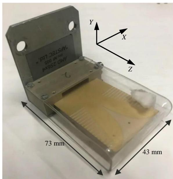
Fig. 3. Vivaldi antenna used in MMSS
