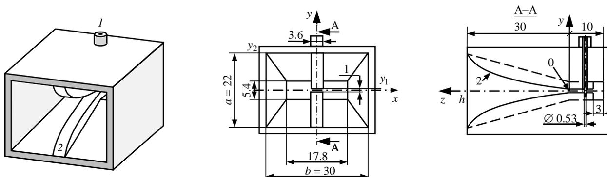
Fig. 4. Double-ridged pyramidal horn model:
