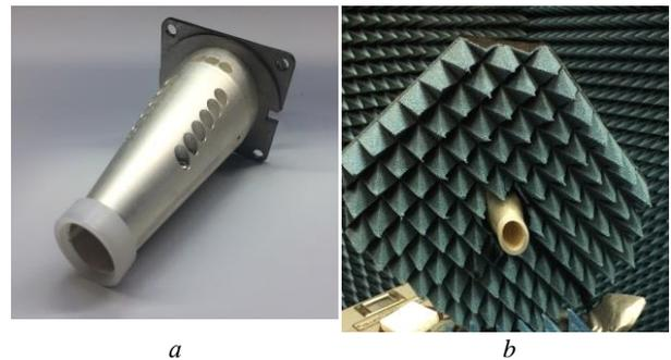
Fig. 11. Elliptical double-beam antenna: *a* – model; *b* – installation in the ECCOSORB VHP-2-NRL absorber array
