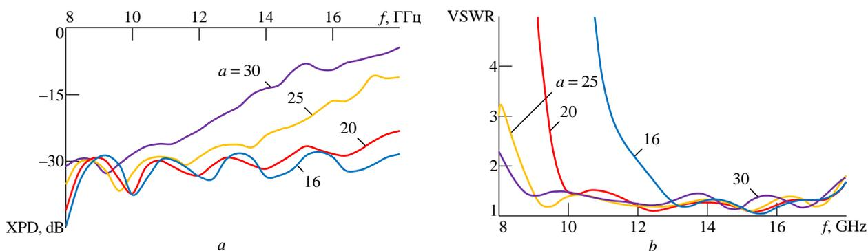
Fig. 7. Frequency dependences of the parameters of the conic horn: *a* – XPD in a spatial angle of 30°; *b* – VSWR
