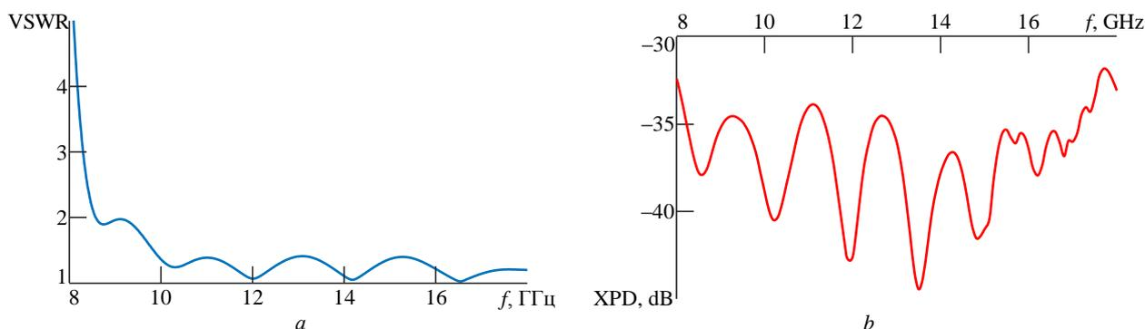
Fig. 9. Frequency dependences of the parameters of the elliptical double-ridged antenna: *a* – VSWR; *b* – XPD in a spatial angle of 30°
