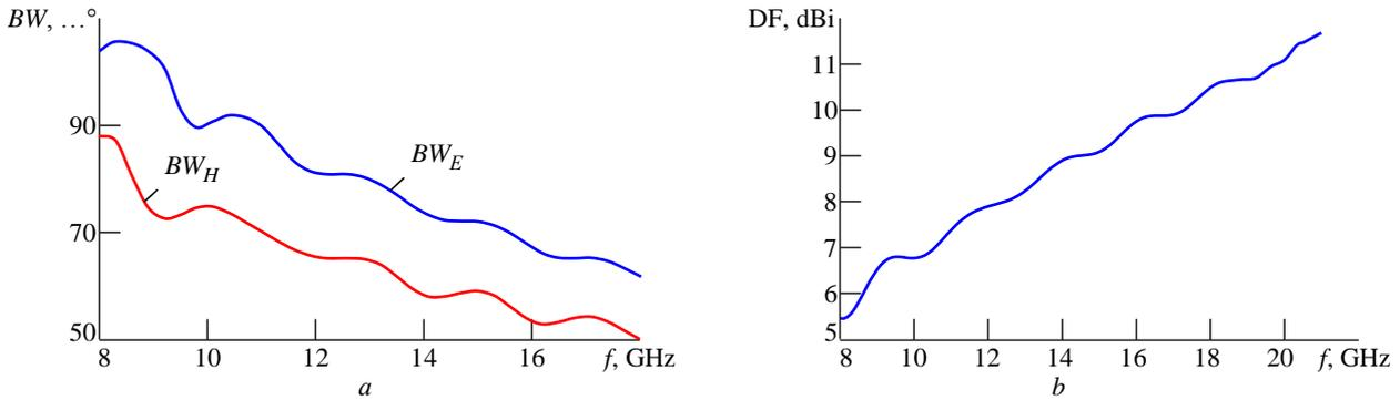
Fig. 10. Frequency dependences of the parameters of the an elliptical double-rib antenna: *a* – radiating pattern by level –3 dB in *E*-plane (blue line) and *H*-plane (red line); *b* – DF
