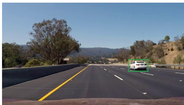
Fig. 1. Visualization of bounding boxes predicted by an object detector, if the probability of finding objects in a rectangle is more than 0.5 ( a ) and more than 0.05 ( b )
