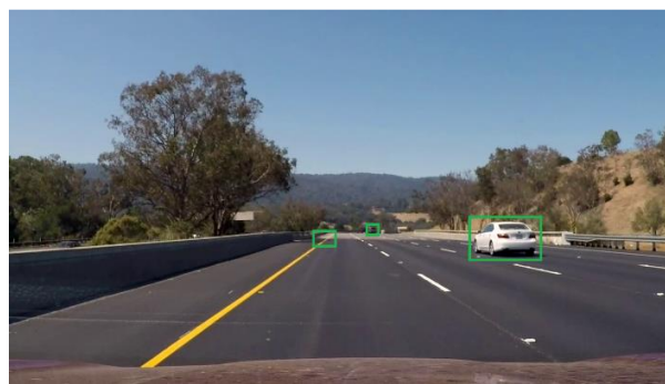
Fig. 1. Visualization of bounding boxes predicted by an object detector, if the probability of finding objects in a rectangle is more than 0.5 ( a ) and more than 0.05 ( b )
