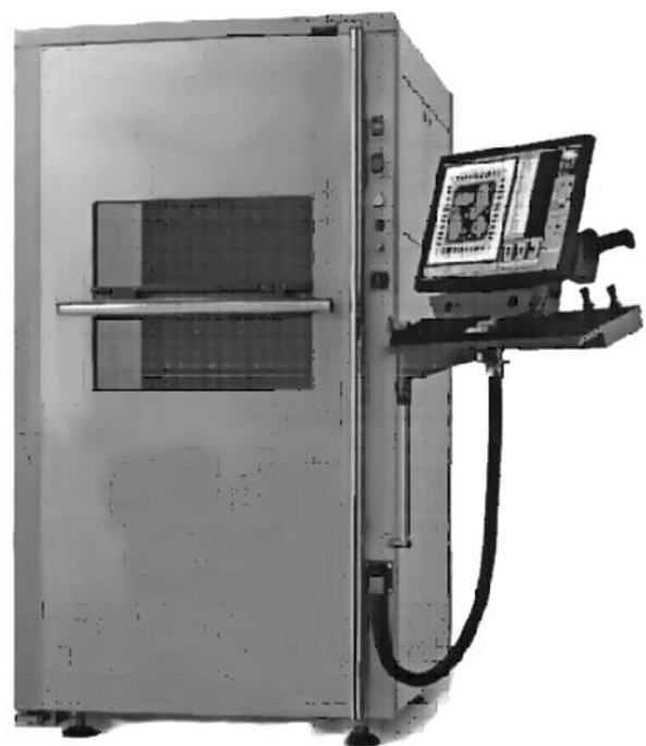
Fig. 2. The example of one of the design implementations of X-ray inspection system of electronic components
